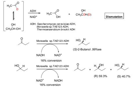
and produces the (S)-alcohol with high enantiospecificity 99%ee.
