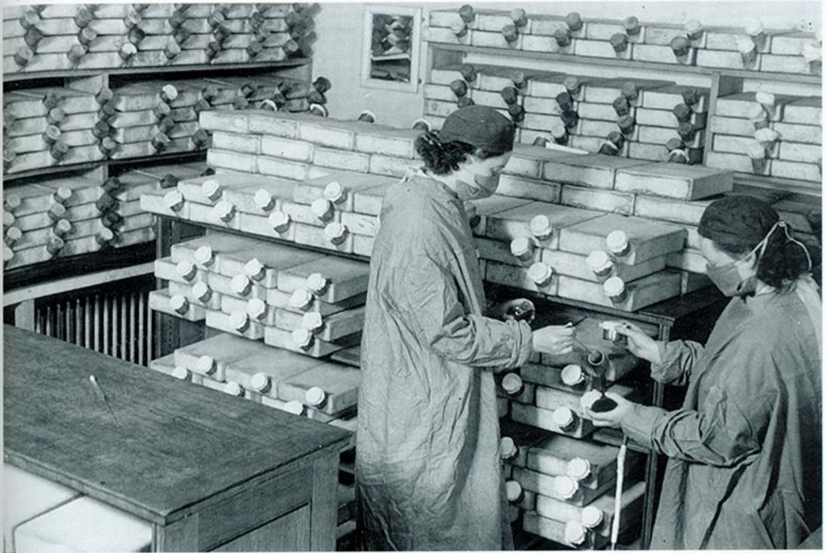
“Penicillin Girls” tending the Heatley-designed vessels for growing penicillin mould at the Sir William Dunn School in Oxford. COURTESY OF NORMAN HEATLEY
