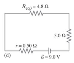
(c) Now we can work back and get the current in the 6.0- $\Omega$  resistor. It must be the same as the current through the 8.7  $\Omega$  shown in Fig. 26–10c (why?). The voltage across that 8.7  $\Omega$  will be the emf of the battery minus the voltage drops across r and the 5.0- $\Omega$  resistor:  $V_{8.7} = 9.0 \text{ V} - (0.87 \text{ A})(0.50 \Omega + 5.0 \Omega)$ . Applying Ohm's law, we get the current (call it I')
