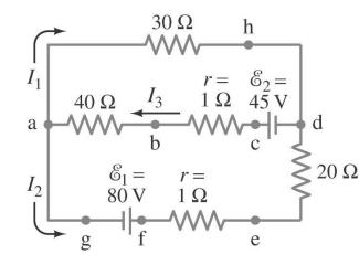
Solve the equations. We have three equations—labeled (a), (b), and (c)—and three unknowns. From Eq. (c) we have
