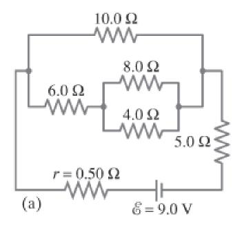
**APPROACH** To find the current out of the battery, we first need to determine the equivalent resistance  $R_{\rm eq}$  of the entire circuit, including r, which we do by identifying and isolating simple series or parallel combinations of resistors. Once we find I from Ohm's law,  $I=\mathscr{E}/R_{\rm eq}$ , we get the terminal voltage using  $V_{\rm ab}=\mathscr{E}-Ir$ . For (c) we apply Ohm's law to the 6.0- $\Omega$  resistor.
