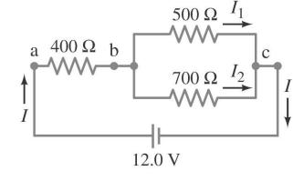
**SOLUTION** The equivalent resistance,  $R_{\rm p}$ , of the 500- $\Omega$  and 700- $\Omega$  resistors in parallel is given by
