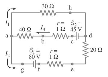
The negative sign indicates that the direction of  $I_1$  is actually opposite to that initially assumed and shown in Fig. 26–13. The answer automatically comes out in amperes because all values were in volts and ohms. From Eq. (d) we have
