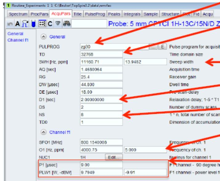
Pulse Program. zg30 means 30° hard pulse, and acquire
