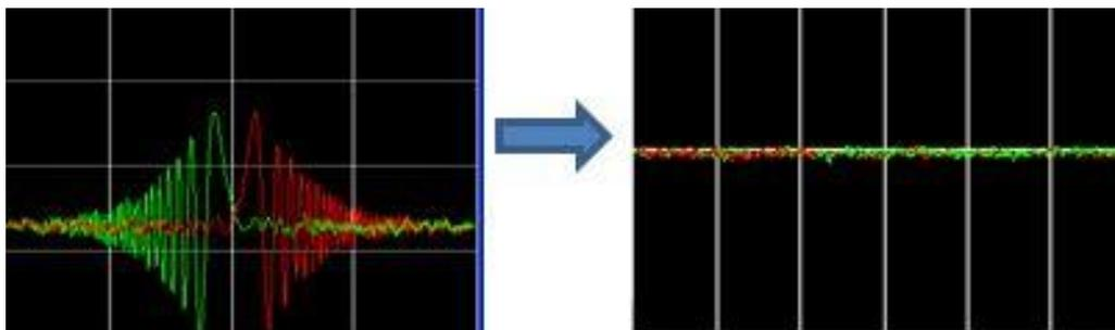
The lock signal can be controlled **manually** by adjusting Phase, Power, Gain, and Field (with lock off). The Field parameter is Z0.
