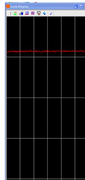
For best resolution, adjust the X, Y and XY shims to obtain the maximum lock level.
