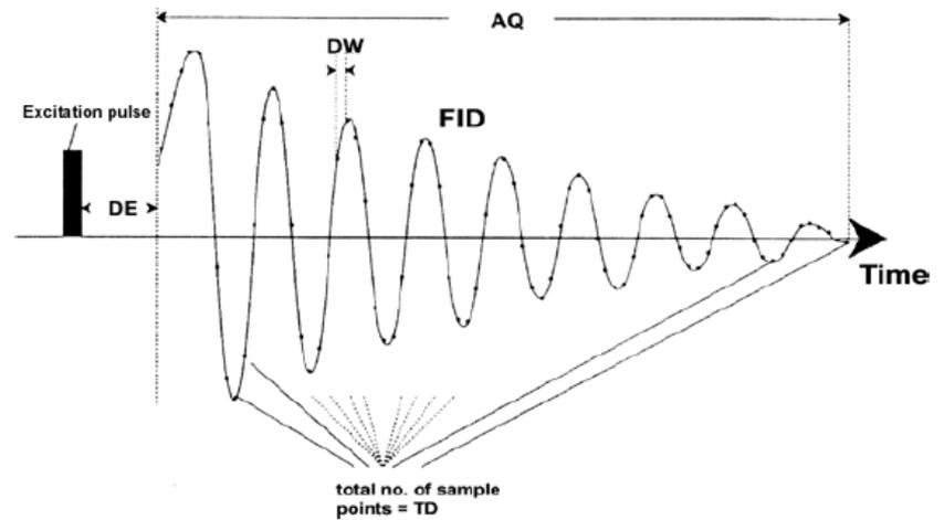
**ns**: number of scans. Increasing the number of scans increases signal-to-noise ratio, but also increases overall experiment time.
