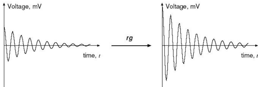
The NMR-signal received from the resonant circuit in the probehead needs to be amplified to a certain level before it can be handled by the computer.
