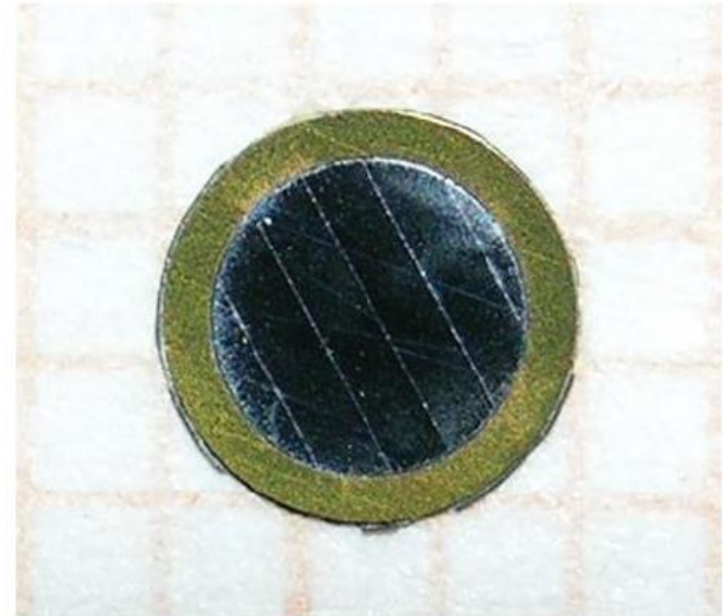
Cross sectional specimen after mechanical polishing
