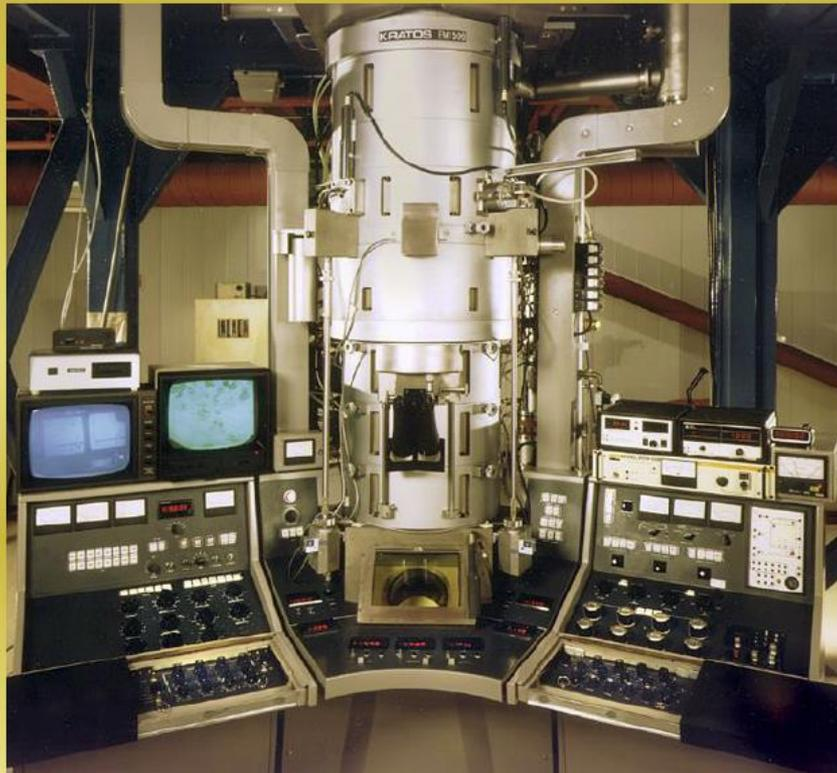
A 1-MeV TEM coupled with a field emission source can achieve resolutions that are in the range of  $0.5\text{\AA}$  !
