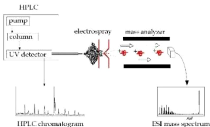
**Figure 3.** Interfacing A) gas chromatography with mass spectrometry and B) liquid chromatography with electrospray ionization mass spectrometry.
