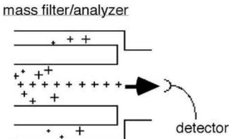
**Figure 19.** After an ion passes through the Mass Analyzer a signal is produced by the detector.
