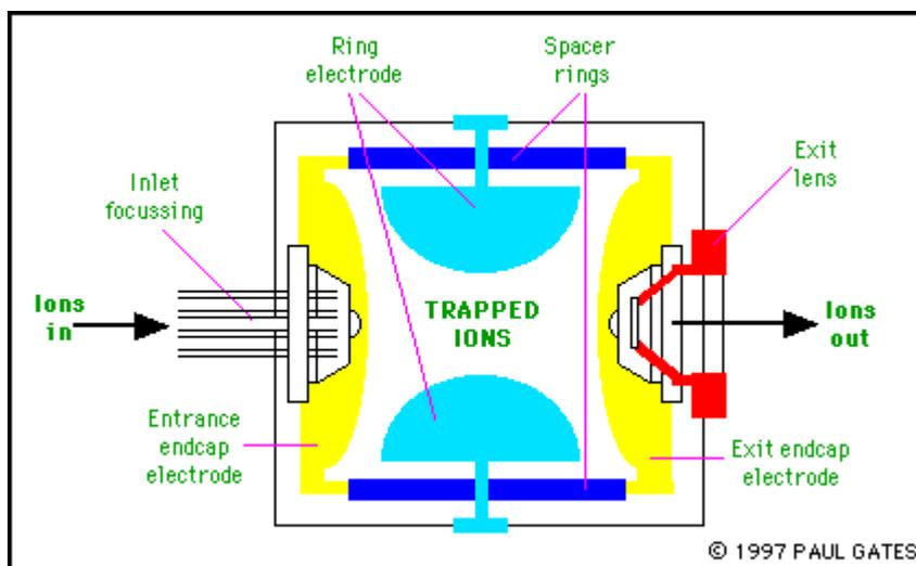
**Figure 16.** A schematic diagram of an ion trap mass spectrometer.
