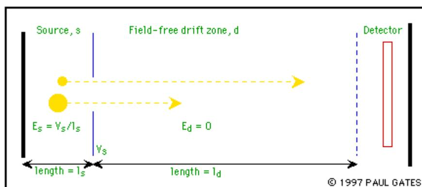
**Figure 13.** Schematic diagram of the process of time-of-flight mass spectrometry: The larger the ion, the slower its velocity and thus the longer it takes to traverse the field-free drift zone. The field in the field-free zone,  $E_d$ , is zero at all times.
