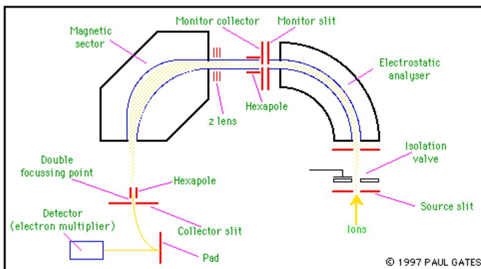
**Figure 11.** A schematic diagram of two-sector mass spectrometer.
