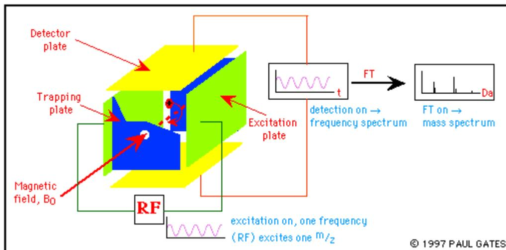
**Figure 15.** A schematic diagram of the trapping, excitation and detection of a ions, to produce a mass spectrum, in FT-ICR mass spectrometry.
