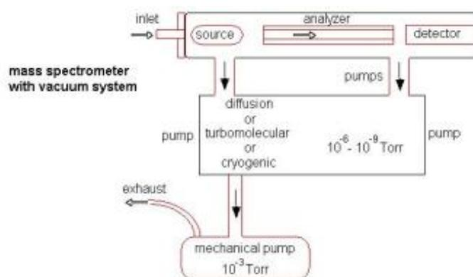
**Figure 2.** A diagram of a Mass Spectrometer outlining the vacuum system.
