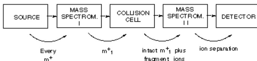
**Figure 17.** Illustration of MS/MS instruments
