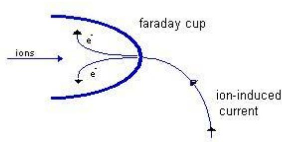
**Figure 20.** Faraday cup converts the striking ion into a current.
