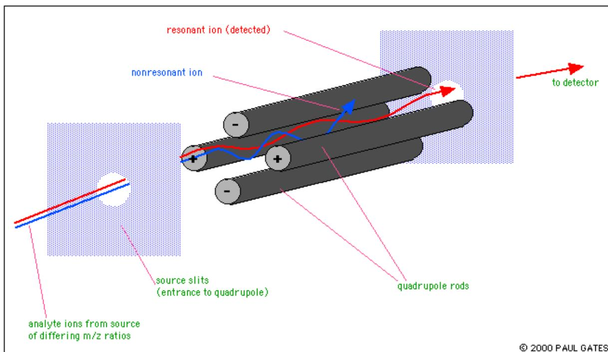
**Figure 14.** Schematic diagram of a quadrupole mass analyser: The four rods are shown as being circular in the diagram but in practice they have a hyperbolic cross-section.
