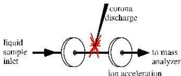
**Figure 7.** Atmospheric Pressure Chemical Ionization (APCI) Mass Spectrometry.
