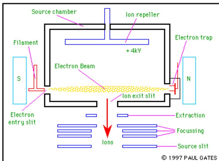
**Figure 4** Schematic of an Electron Ionization (EI) Source
