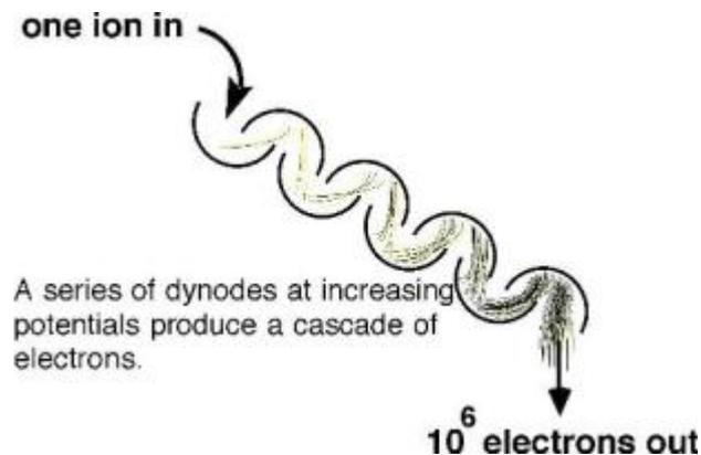
**Figure 21.** Electron multiplier and the cascade of electrons that results in a factor of one million signal amplification in a mass spectrometer.
