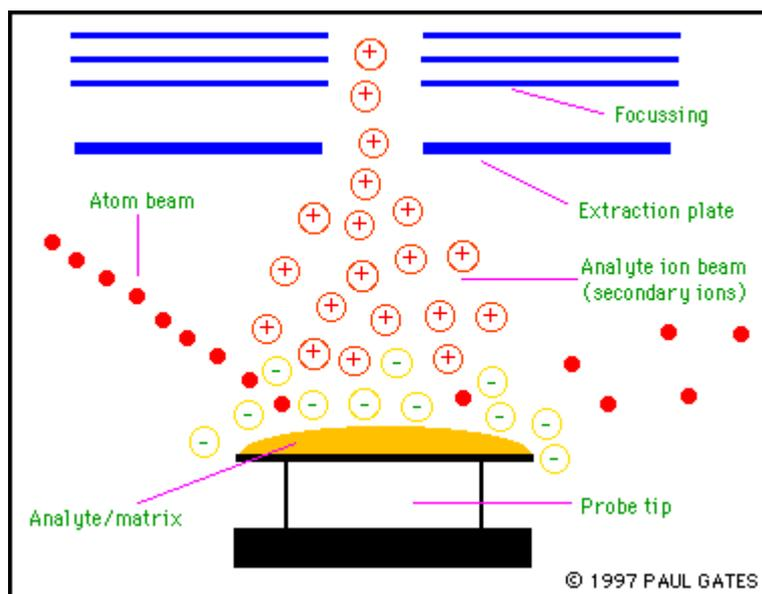
**Figure 5.** Schematic of a Fast Atom Bombardment source (positive mode).
