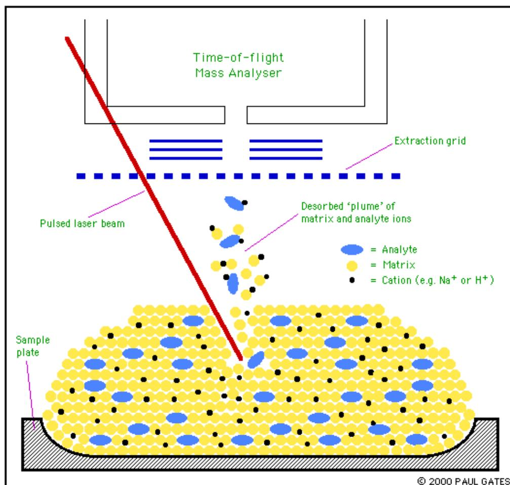
**Figure 8.** Schematic of MALDI
