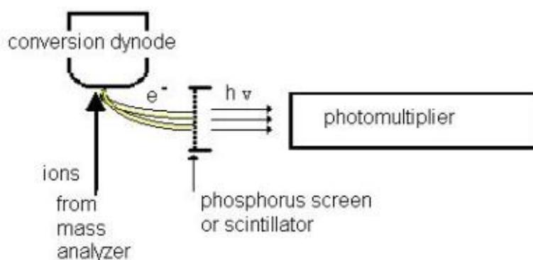
**Figure 22.** Scintillation counting relies on the conversion of the ion/electron signal into light. Once the photon(s) are formed, detection is performed with a photomultiplier.
