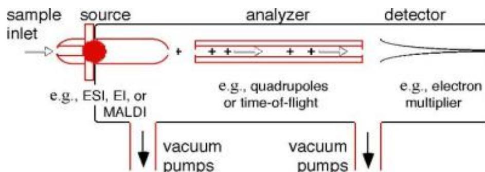
Figure 1. Components of a Mass Spectrometer
