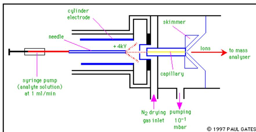
**Figure 6.** A schematic diagram of the typical layout of an electrospray source.
