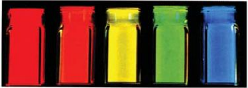
Figure 20.1. Color photographs of cadmium selenide nanoparticles illuminated with a long-wave UV lamp. Revised from [2].
