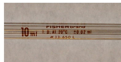
Figure 4.2 Close-up of a 10-mL volumetric pipet showing that it has a tolerance of \pm 0.02 mL at 20 °C.
