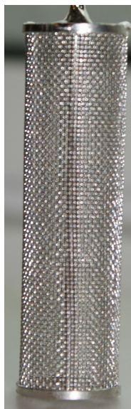
Figure 11.29 Example of a cylindrical Pt-gauze electrode used in controlled-potential coulometry. The electrode shown here has a diameter of 13 mm and a height of 48 mm, and was fashioned from Pt wire with a diameter of approximately 0.15 mm. The electrode's surface has 360 openings/cm 2 and a total surface area of approximately 40 cm 2 .
