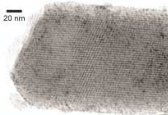
c -C 20 PyPt 3 SnSe particle viewed down the [110] cubic plane.
