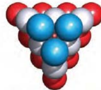
Layer A (red spheres) Layer B (grey spheres) Layer C (blue spheres)
