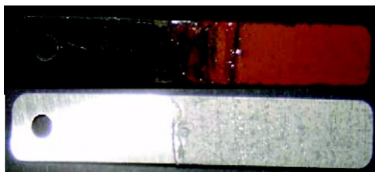
Figure 11. Corrosion protection by Zn-HDTMP (control, upper; inhibited, lower).
