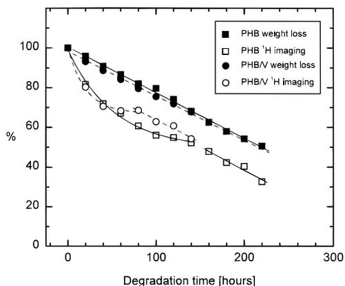
**Figure 4.** Total weight loss (%), and <sup>1</sup>H image integral loss (%) of degraded PHB and PHB/V as a function of degradation time by PHB depolymerase B from *P. lemoignei*. The curves for the initial <sup>1</sup>H imaging data (PHB, 0–140 h; PHB/V, 0–80 h) are single exponential fits, all others are linear fits. For parameter values see text and Table 1.
