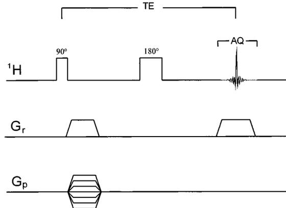
**Figure 1.** Spin-echo pulse sequence used for the <sup>1</sup>H NMR imaging experiments.  $G_r$  and  $G_p$  are the read and phase gradients respectively, AQ is the acquisition time, and TE is the echo time.
