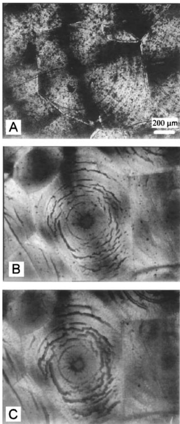
**Figure 5.** Polarizing optical micrographs of a melt cast PHB film: (A) No degradation; (B) 20 h of degradation by PHB depolymerase B; (C) 40 h of degradation. Notice the increasing width of the erosion patterns from part b to part c and the characteristic hole in the spherulite center.<sup>13,18</sup>
