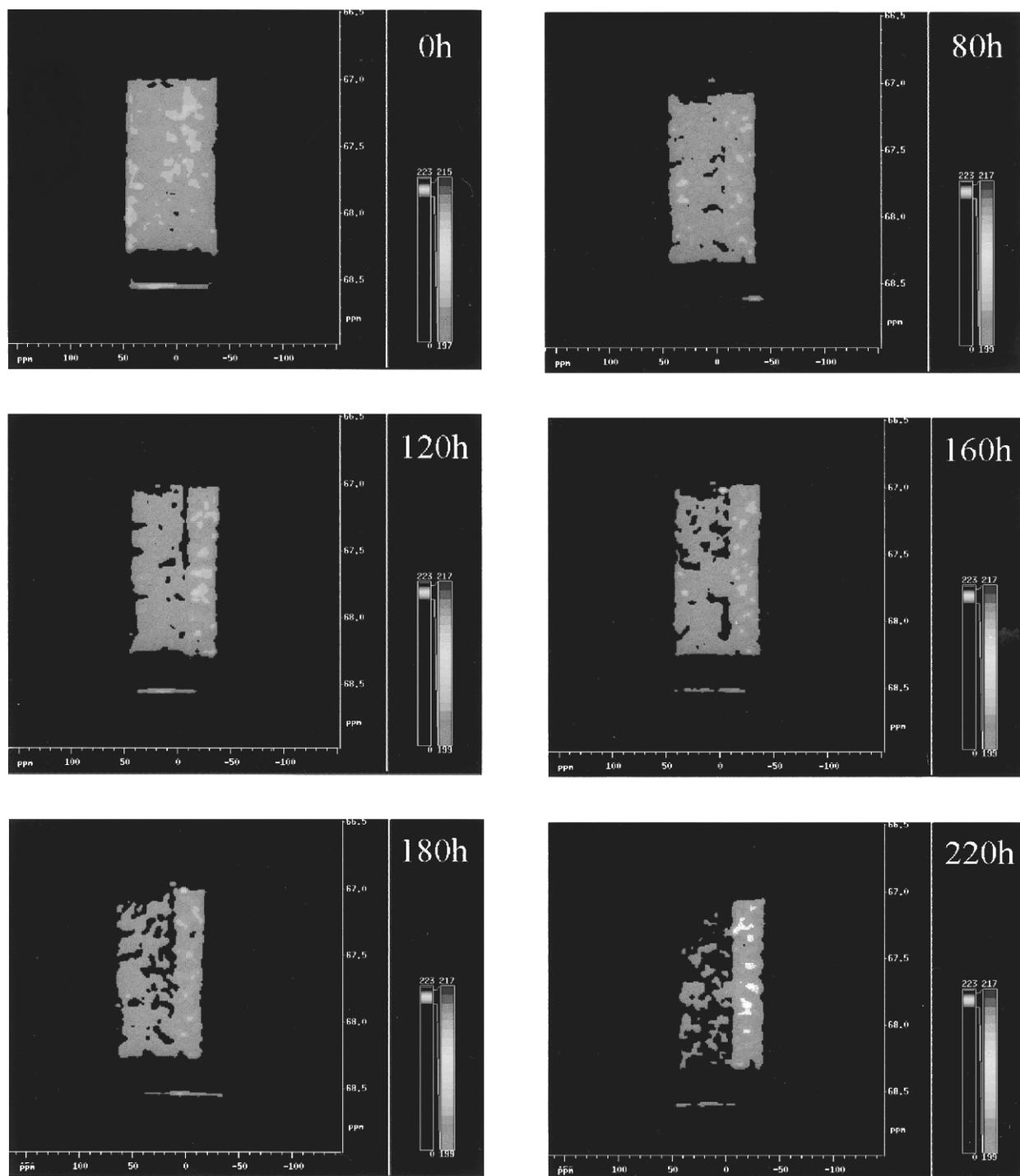
**Figure 2.**  $^1\text{H}$  NMR images of a PHB film (large piece of film on the left), as a function of degradation time indicated at the top right of each image (FOV  $3 \times 3 \text{ cm}^2$ ). A smaller but identical never degraded piece of PHB film, used as a standard, can be seen at the right of the degraded one in all images. The small intensity appearing at the bottom of the images comes from the Teflon sample holder.
