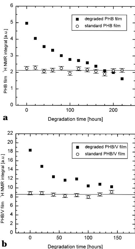
**Figure 3.** Variation of the integral values of the <sup>1</sup>H images of a degraded PHB film (a) and a PHB/V film (b) as a function of degradation time at 37 °C by PHB depolymerase B from *P. lemoignei*. The integrals of the never degraded standard PHB and PHB/V films are also shown in each graph. The lines are drawn across the mean value obtained for the standard, 2.12 and 8.57 au for PHB and PHB/V respectively.
