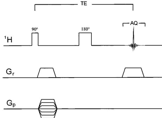
**Figure 1.** Spin-echo pulse sequence used for the  $^1\text{H}$  NMR imaging experiments.  $G_r$  and  $G_p$  are the read and phase gradients respectively, AQ is the acquisition time, and TE is the echo time.
